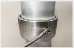
The **PN100** connection from GWE is a riser pipe connection with a particularly robust design based on established ZSM technology. Designed for high pressure levels, the system achieves its high tensile strength via two link chains instead of conventional shear rods.
